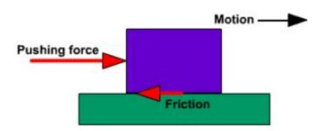
'Friction' is a force that resists motion of sliding or rolling of one object moving relative to another. It is a result of the electromagnetic attraction between the charged particles of two touching surfaces. We find and use it everywhere and every day whenever objects come into
