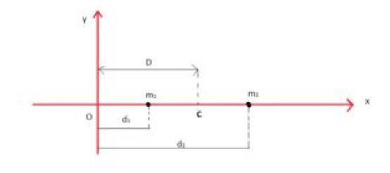
In the figure above, we take two particles with masses m<sub>1</sub> and m<sub>2</sub> respectively lying on the x-axis. The distance of both the particles from the centre O is d<sub>1</sub> and d<sub>2</sub> respectively. The CoM of this two system of particles is at point C lying at a distance D from point O. In this system of two particles D can be written as:
