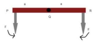
The figure shows an instance of rotational equilibrium. Q being the center with sides PQ=QR=a. The forces F at points P and Q are equal in magnitude but opposite in direction. The system is in rotational equilibrium as the net moment on the rod is zero. The translational
