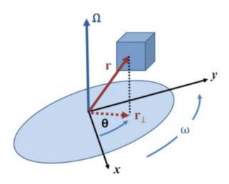
Consider a particle of mass m at a distance from the axis with linear velocity =  $v_i = r_i \omega$ . Therefore, the kinetic energy of this particle is,
