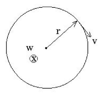
Angular velocity =  $\omega \times r$ . The second hand of the clock rotates in clockwise direction. From the above figure, the direction of angular velocity is into the plane of the page that is inward towards the clock face.
