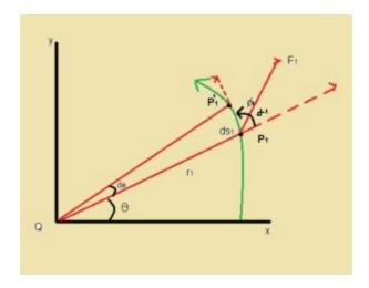
The graph above represents work done by a torque acting on a particle that is rotating about a fixed axis. The particle is moving in a circular path with center Q on the axis. P1P'1 is the arc of displacement ds1. The graph in the figure shows the rotational motion of a rigid body across a fixed axis.
