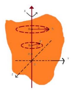
The figure above shows a rigid body's rotation along a fixed axis. Here the axis on which the rotational motion occurs is the X-axis. If P1 is a particle of the rigid body's system moving with its center D1 on the fixed axis then the circular plane in which the motion takes place lies in a plane that is perpendicular to the X-axis. The same situation is with another particle P2. Here both these particles move in a circular motion with their respective radius r1 and r2 at centers D1 and D2.
