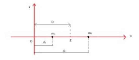
In the figure above, we take two particles with masses m<sub>1</sub> and m<sub>2</sub> respectively lying on the x-axis. The distance of both the particles from the centre O is d<sub>1</sub> and d<sub>2</sub> respectively. The CoM of this two system of particles is at point C lying at a distance D from point O. In this system of two particles D can be written as:
