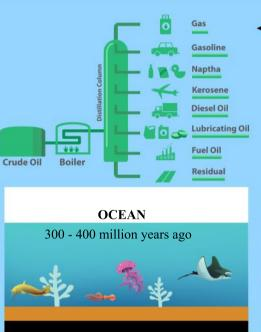
Is a mixture of many liquids which are separated by fractional distillation as they have different boiling points
